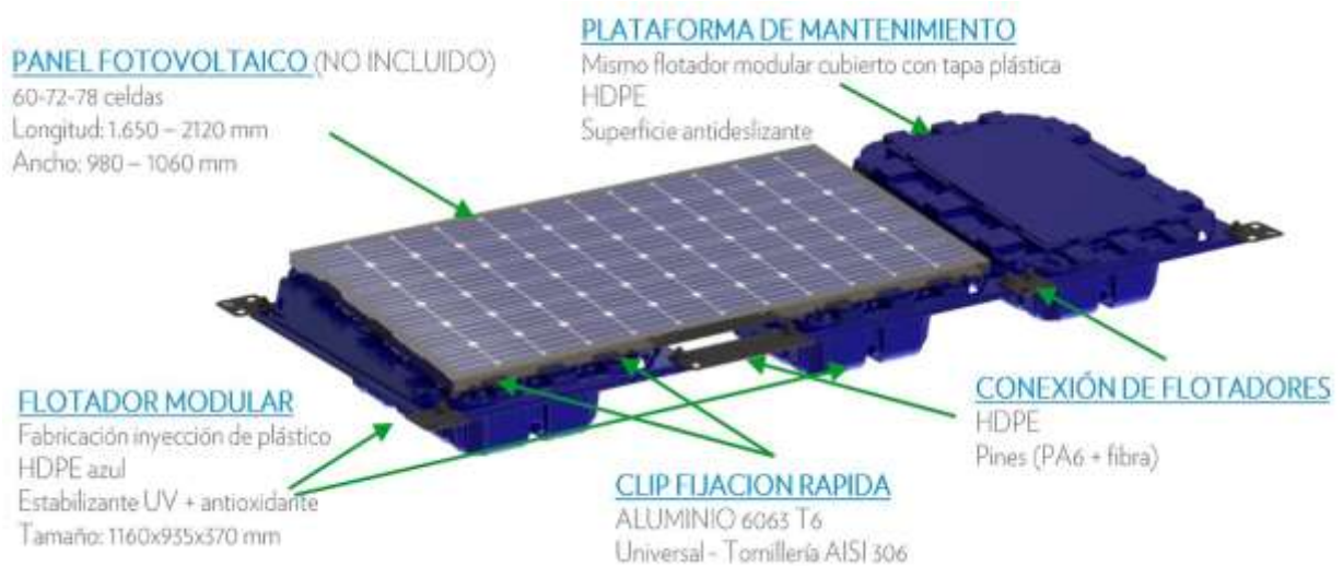
Figure 12: Design specifications of the Spanish Isifloating modular floats to support photovoltaic panels
