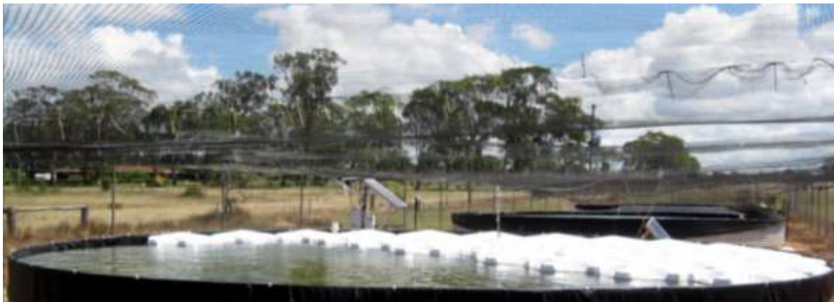
Figure 11: Floating modules drifting across a 10 m diameter tank in Toowoomba.
