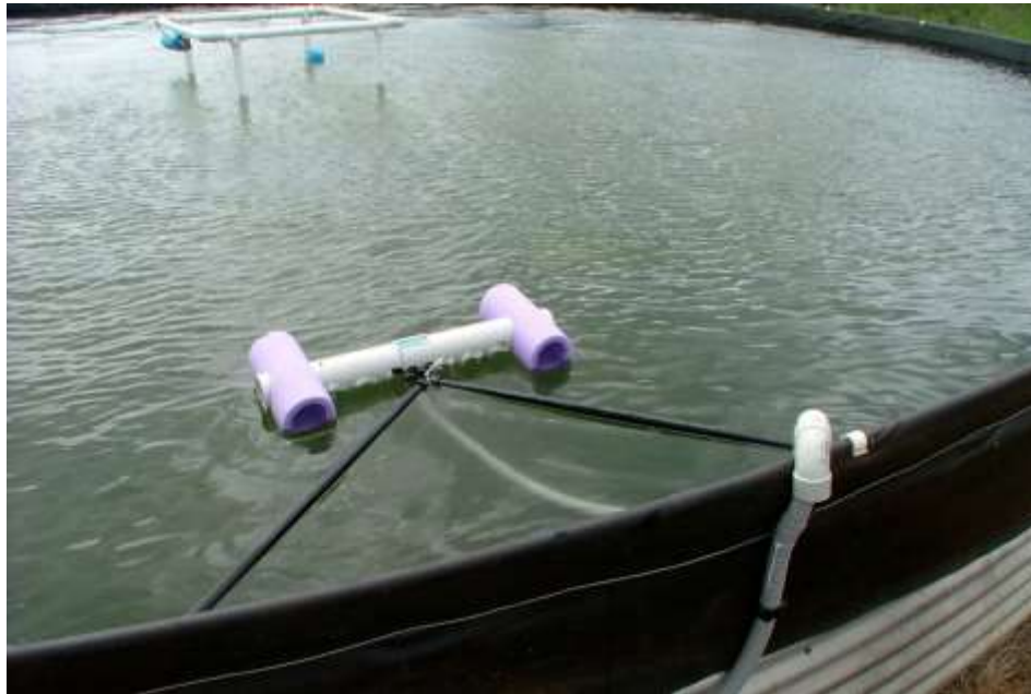
Figure 15: Sampling the microlayer from under a suspended cover
