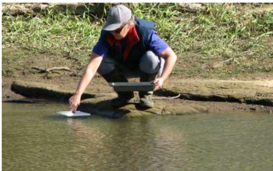
Figure 16: Sampling the microlayer with a perforated, Teflon plate
