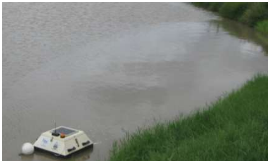
Figure 14: Experimental compound C18E1 spreading from an automated applicator on a brown water storage (Logan's Dam, Lockyer Valley) during monolayer application.
